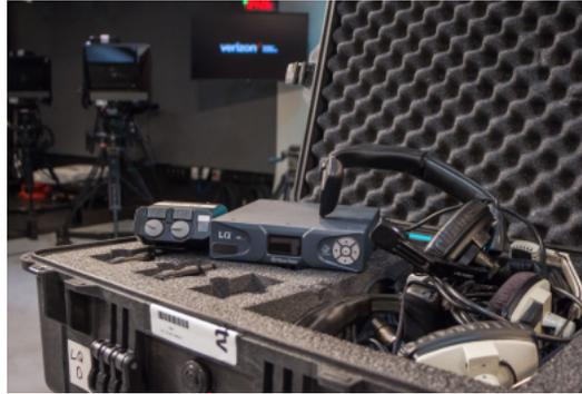
Verizon sends out pre-configured fly packs of Intercom gear to each location participating in a particular corporate production. Crews use RTS headsets and belt packs in tandem with a Clear-Com LQ IP interface unit.
