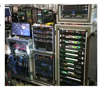
Inside the KeyArena were dozens of video screens, specialty mood lighting controllers, sound systems, and other electronic devices. Many of these are electronically noisy and produce unwanted electrical artifacts that can be a problem for analog communications.
