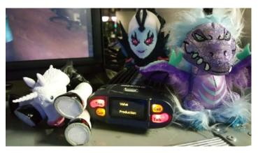
Due its all-digital design, HelixNet is impervious to noise, hum, or other problems that might exist in analog-based intercom systems. HelixNet also does not generate any unwanted electrical artifacts within itself, so the intercom system did not disrupt any of the electronic products in use by the gamers.
