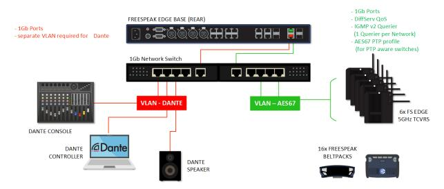
In this scenario you will split the LAN connections on the FS Edge/Arcadia Station to ensure LAN X is only used for connection to the FreeSpeak IPT network with LAN Y only used for connection to the Dante audio network. LAN X and LAN Y **must not** be connected to the same VLAN.
