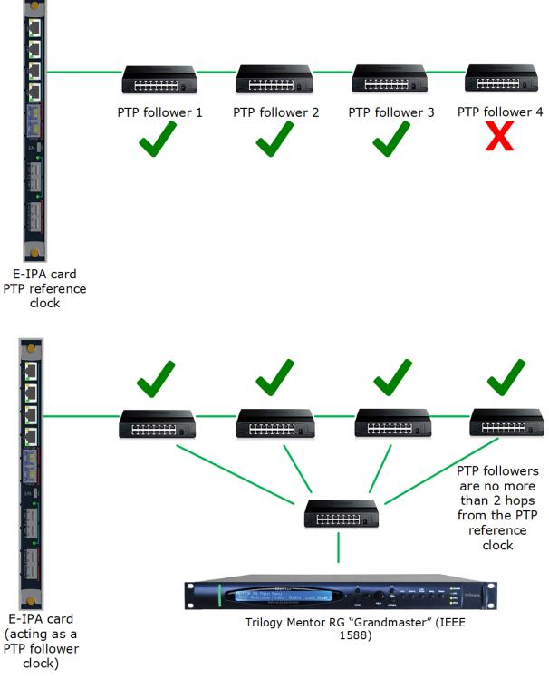
Note: in this configuration, RSTP/STP needs to be enabled
