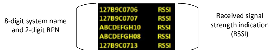
Figure 3-4 An unconnected beltpack site survey screen
