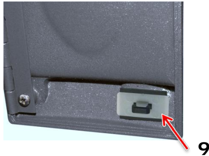
Figure 2-7: Removing the white plastic protector from the latch
