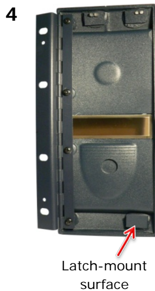
Figure 2-4: Latch-mount surface, inside the Eclipse HX door
