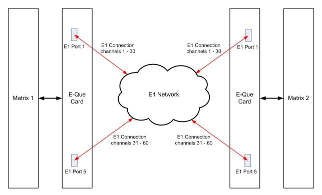
The E-QUE interface can also be used to connect the matrix to third party equipment using E1 port 1 or 5.
