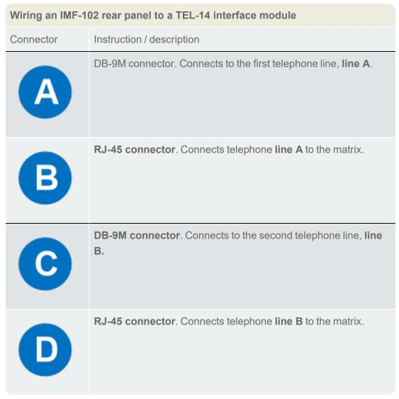
**Note**: To allow use of a common RJ-11 terminated telephone line, Clear-Com provides two DB-9F to RJ-11 adapters (Clear-Com part 770025)
