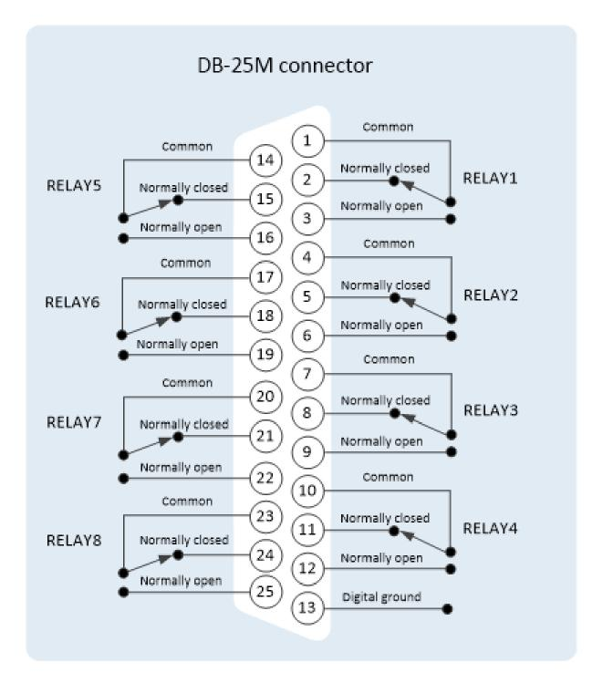
**Note** The general purpose outputs are single-pole double-throw relays with contact ratings of 30 VDC (volts direct current) at 1 ampere.
