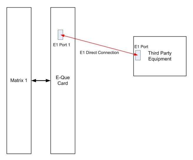
The CAT5 cable connecting the E1 port on the E-QUE rear card may be a crossover cable or a straight-through cable depending on the requirements of the third-party equipment. The E-Que interface should be set to **Direct** in EHX.
