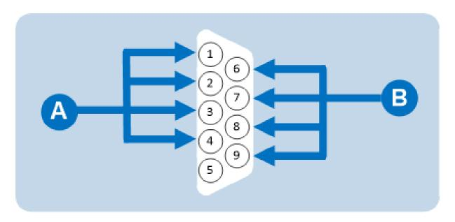
The two DB-9M connectors are paralleled such that both partyline channels are available on each connector. It is possible to:
