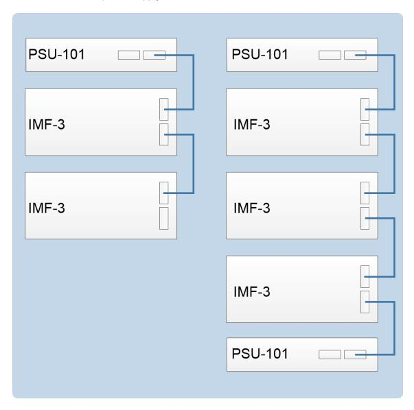
Installing **two** PSU-101 power supplies for each IMF-3 provides redundancy, because either of the two PSU-101 power supplies can power a complete system.
