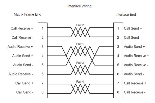
For Eclipse HX-Omega, Eclipse HX-Median and Eclipse HX-Pico, if the GPI/RLY port is used a ferrite core must be added to the socket end of the cable. A suitable ferrite core is **Würth Electronik part 74271132**.
