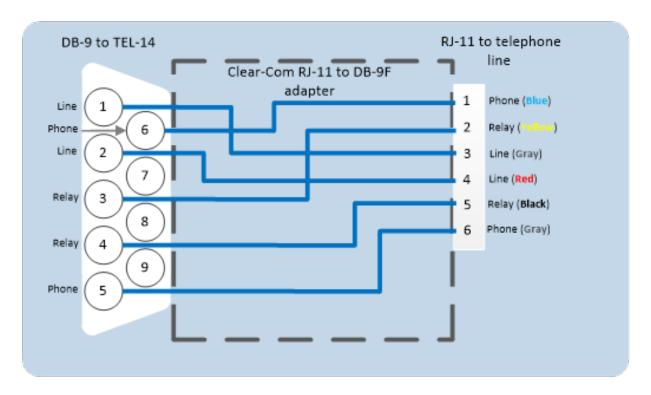
**Note:** The TEL-14 interface works with telephone company central office (CO) lines. Analog panel lines from some in-house PABXs are not compatible.
