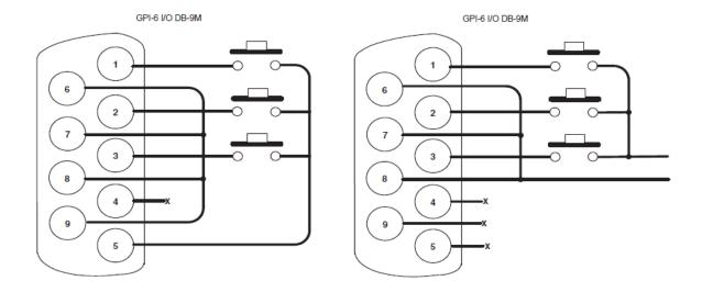
The image above shows you how to connect switches or contacts using the power source provided by the GPI-6 module or powering switches from external sources. Each input can be wired to be isolated from each other as a further variation.
