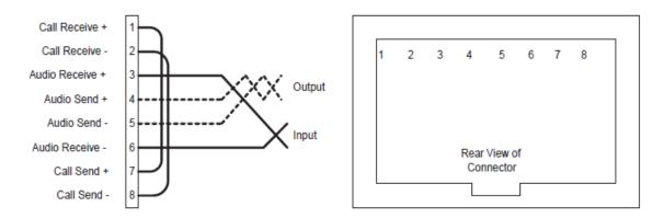
Note: Shielded cable should be used where possible.
