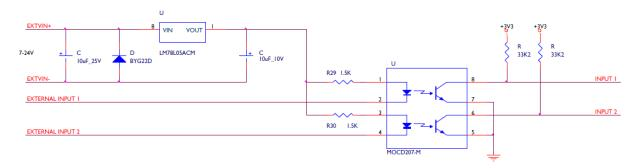
In this mode, a DC voltage of between 7 and 24 volts is required at the **EXTVIN+ pin** with relation to the **EXTVIN- pin**. To cause an input to detect an active signal, current must flow from the relevant input pin.
