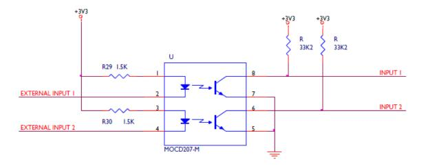
To cause an input to detect an active signal, current must flow from the relevant input pin.
