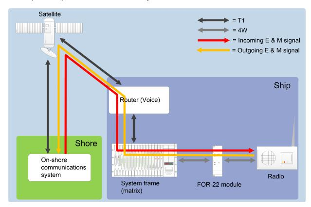
In the image above, E & M signaling is carried with audio channels on the direct T1 connection and then split into logic functions in the matrix:
