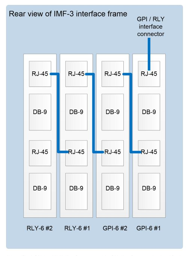
**Note**: If both GPI-6 and RLY-6 interfaces are used the GPI-6 interfaces must be placed first in the daisy chain
