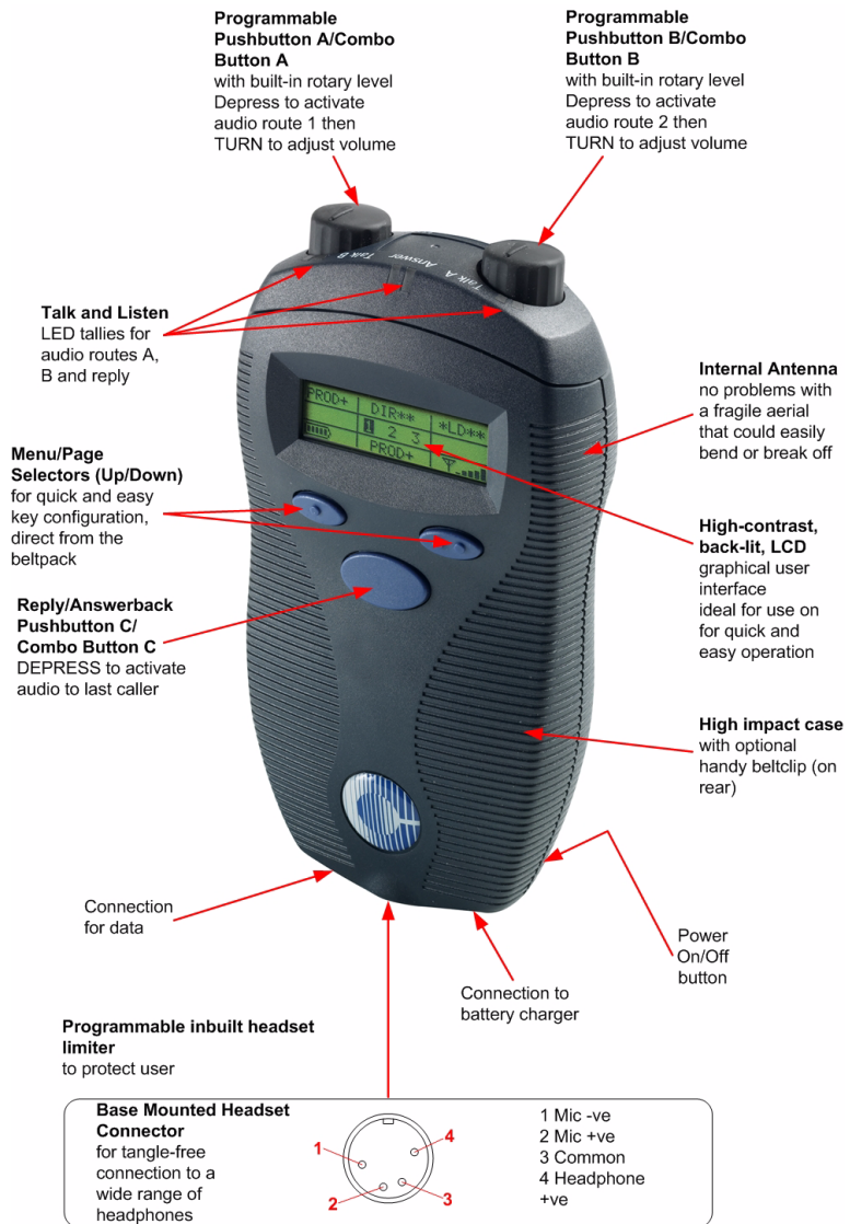
Figure 2-3: Overview of Beltpack Operation
