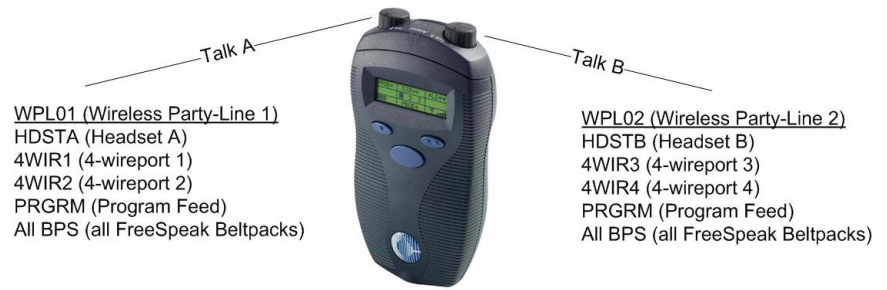
Figure 1-5: Beltpack Configuration with the Default Map
