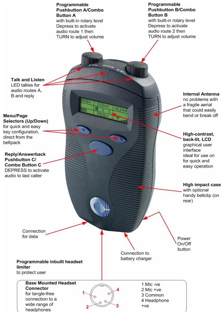
Figure 6-1: Overview of Belt-pack Functions
