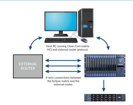
The Host PC receives routing information from the external router and translates this into the appropriate matrix HCI commands that are required to follow the external router actions. Similarly, the Host PC receives routing information from the Eclipse matrix and translates this into the appropriate external router commands. All request messages from the Host have a corresponding reply message from the matrix.
